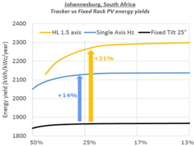
Figure 3: Plant ground coverage ratio (PV array area / land area used)
